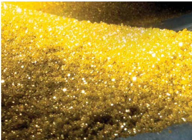
Element Six creates the synthetic diamond that forms the basis for micron, which gives us a high degree of control over crystal size, strength, shape, purity and durability.
